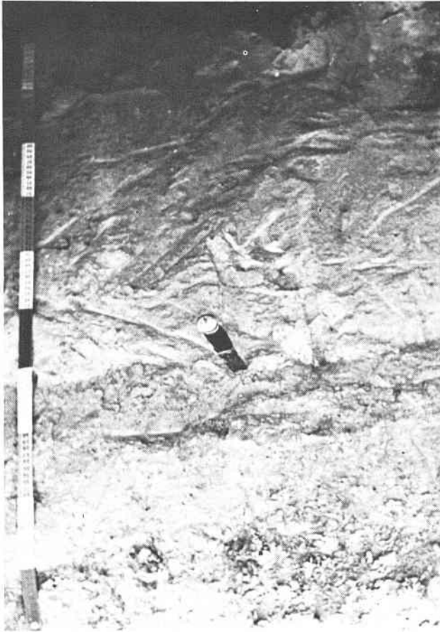
A gypsiferous soil in the Euphrates valley, Syria. The surface contains less than 1 %; the gypsum content below a depth of 37 cm is 45 % (see description profile no 2 in Annex).
