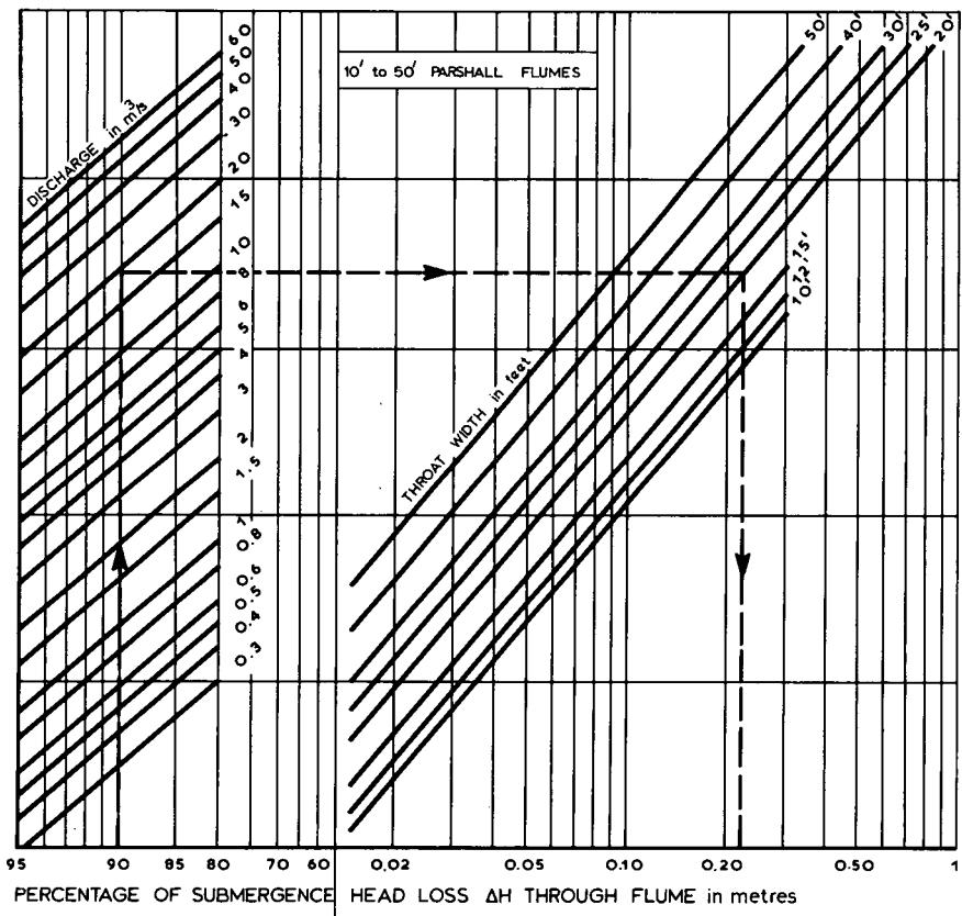
Figure 7.20 Head-loss through Parshall flumes (10-50 feet wide)
